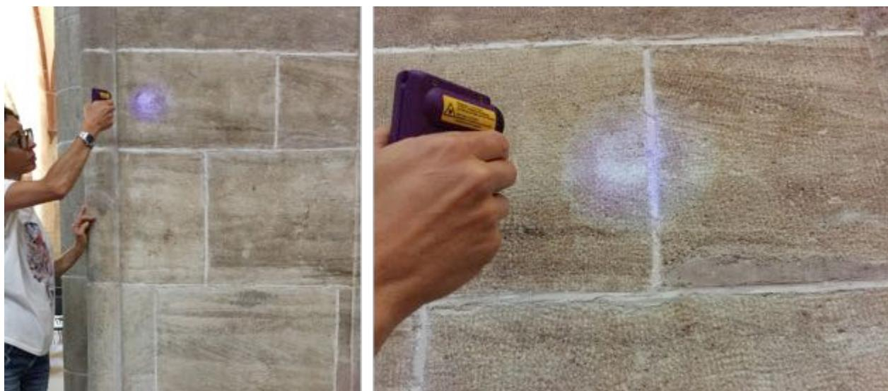
Figure 5.1: Visualisation of traces of organic binder using a UV-light pocket lamp: area presenting UV-fluorescence (dark violet areas) correspond to zone where organic binders are still present.
