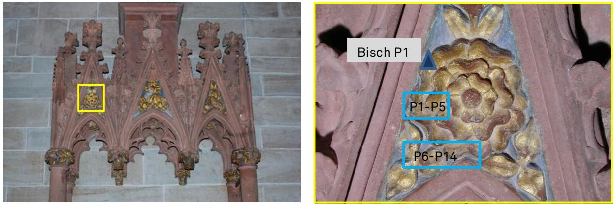
**Figure 3.57:** Localisation of the XRF (ARTAX) analyses and of sample “Bisch P1” on the canopy.
